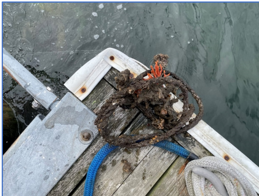
Photograph 1: Typical condition of broken line where anchor connection is located
