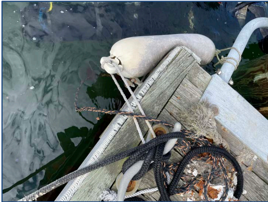
Photograph 3 – 3/8" line broken where anchor attachment location is marked
